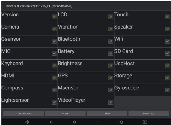
In factory, you can test the corresponding peripheral according to this interface. Click "TEST CHECKED" to test the items one by one. If succeed, click pass, if fail, click failed, the final result will display on the screen, as shown below. Red means failed item, others are pass, and the factory can repair accordingly based on the test result. Besides, if customers need to customize the tool, please contact FAE to apply for the corresponding source code.
