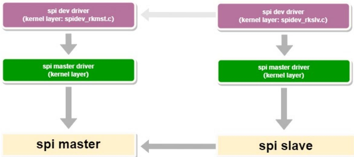
The purpose of providing "SPI Slave Software In Kernel" is to provide reference for protocol and device drivers, and the end customer should also define their product requirements on the application buffer of the slave end to achieve business.
