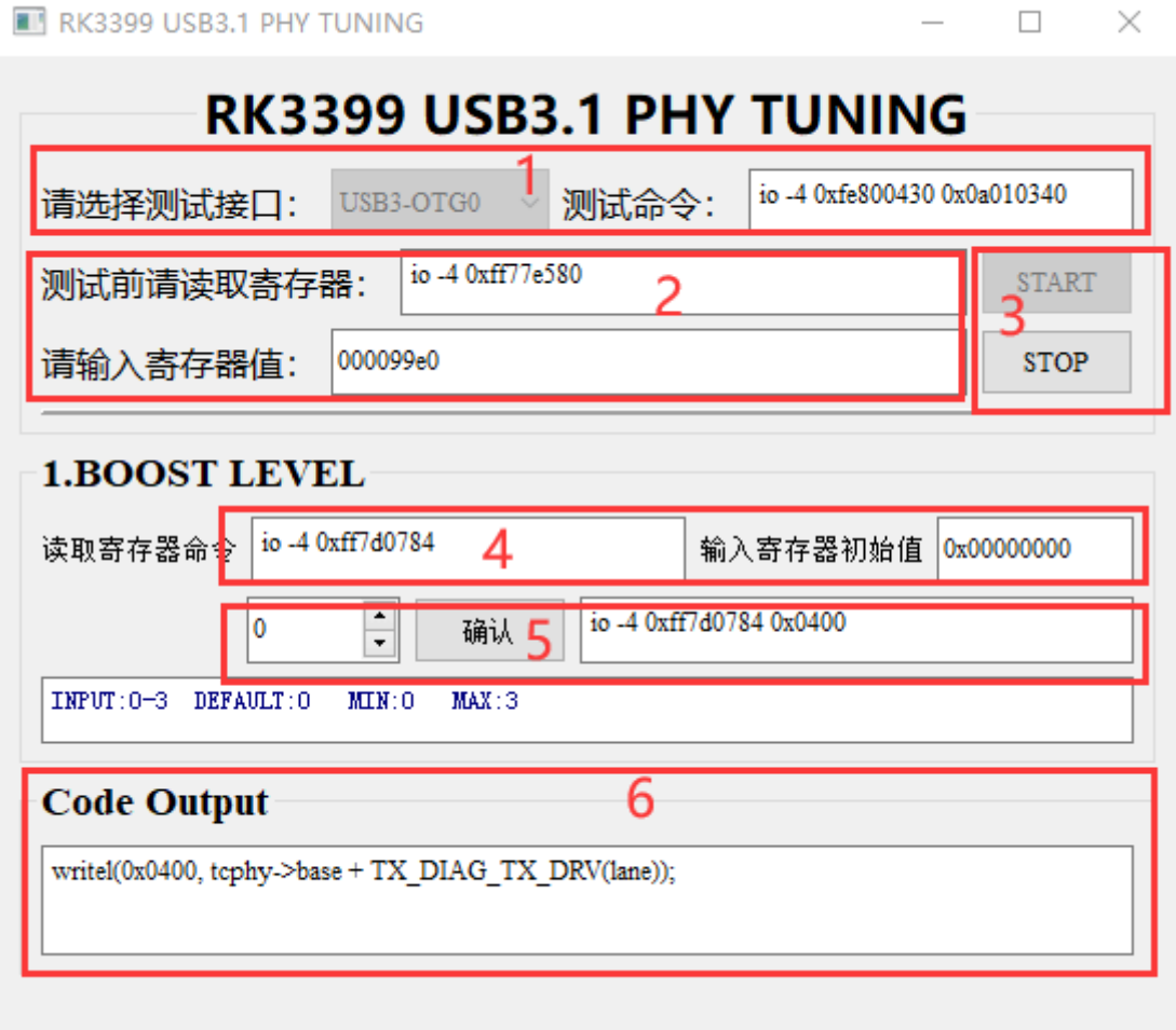
图10 RK3399 USB3.1 PHY Tuning Interface
