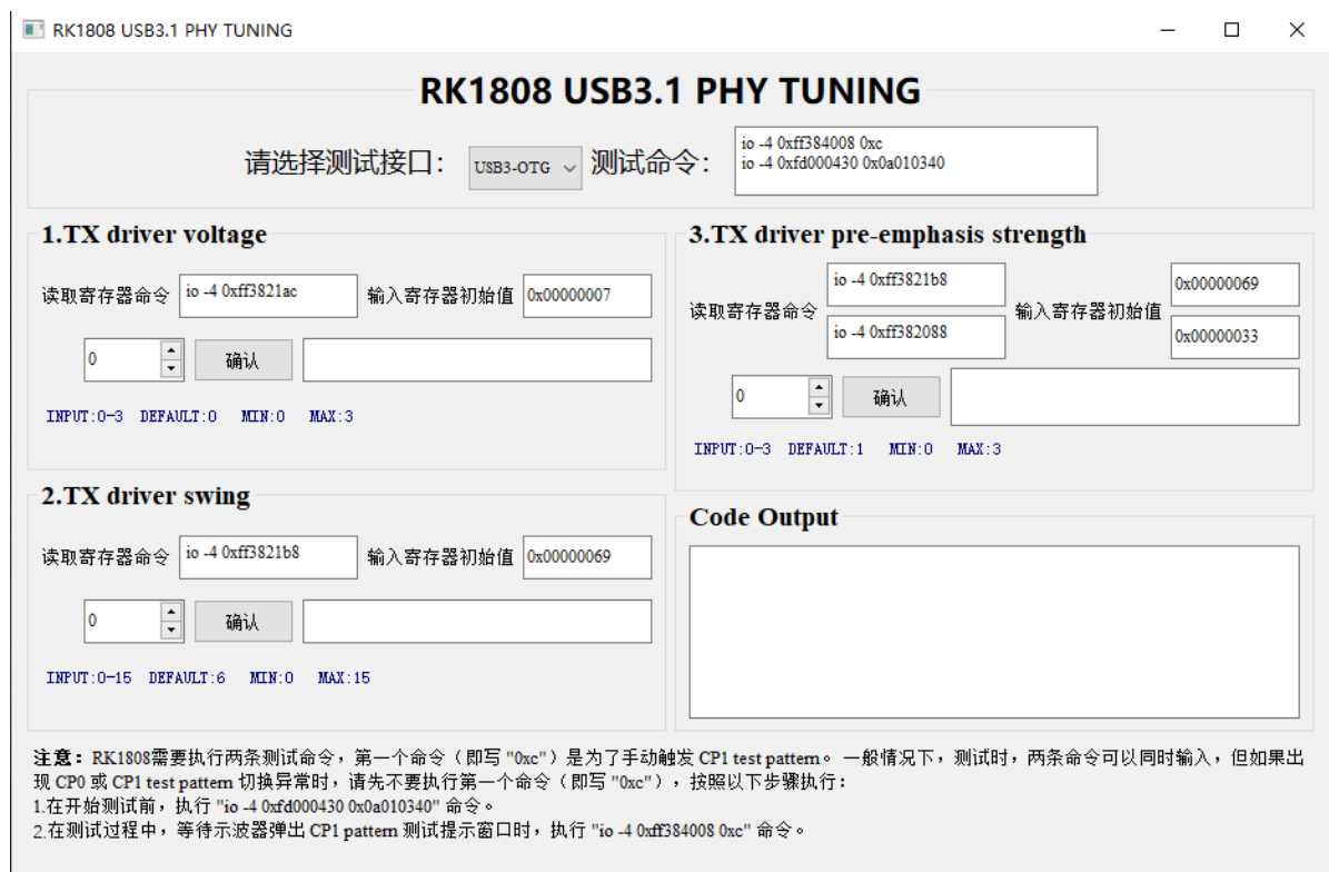
图9 RK1808 USB3.1 PHY Tuning Interface
